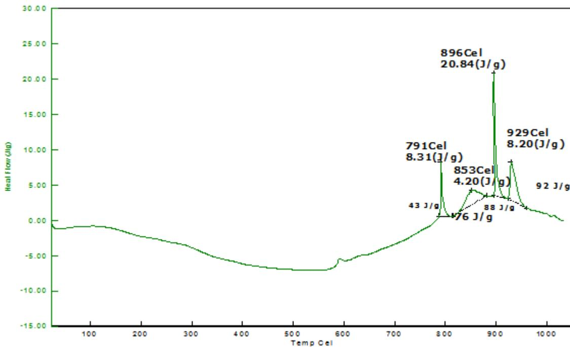
Figure 2 DSC curve of Amorphous Fe<sub>76</sub>Tm<sub>4</sub>B<sub>20</sub> alloy at a heating rate of 20<sup>0</sup>C/min.
