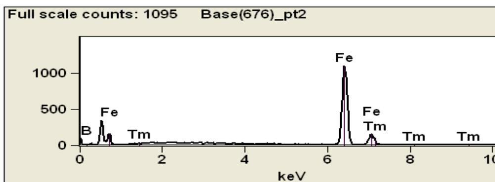
Fig.14 (b) EDS spectrum of the heated sample (S2)
