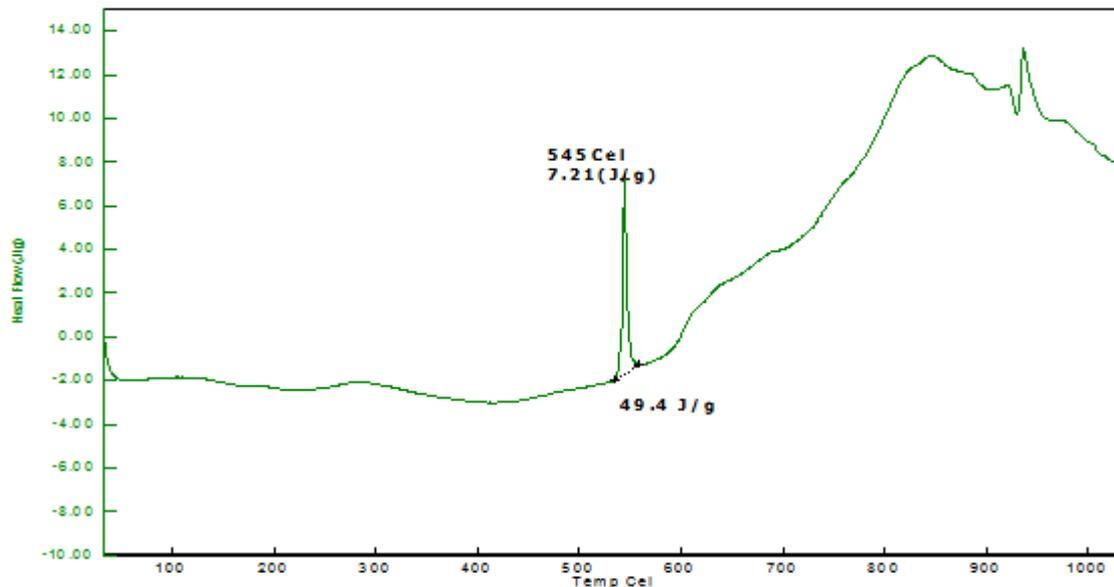
Figure 1 DSC curve of Amorphous  $Fe_{78}Tm_2B_{20}$  alloy at a heating rate of  $20^{\circ}C/min$ .
