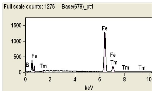
Fig. 12 EDS spectrum of the sample (S1)
